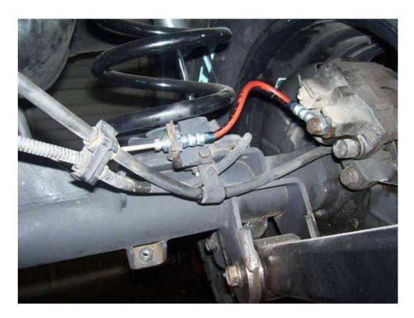
\* Pictures shows Brake line, E-brake cable, And ABS sensor wire routing.
