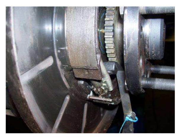
• Picture shows placement of feeler gauge with proper spacing. Also notice round nub on backside of speed sensor this is where tone ring needs to be aligned.
