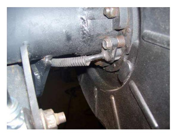
Picture shows metal spacer installed with longer supplied bolt.
