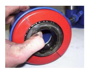
Notice how the bearing is captured by the halves.
