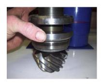
Choose best suited clamshell and slide it under the bearing cage. Proper clamshell size should fit as tight as possible while still allowing the clamshell halves to come together. Then screw the top adjuster upward until it is tight to the top of the clamshell. There should now be no movement up or down when you lift up on the tool.
