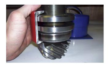
Slide the other clamshell half over the adjuster rings, and slide the locking collar down, set the lock screw to keep the halves from pushing apart.
