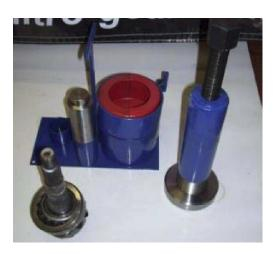
The trick to this tool is the clamshell halves grab the cage of the bearing while the race holds equal pressure on the cage allowing you not to deform the cage or damage it. Assemble the diff puller as shown.
