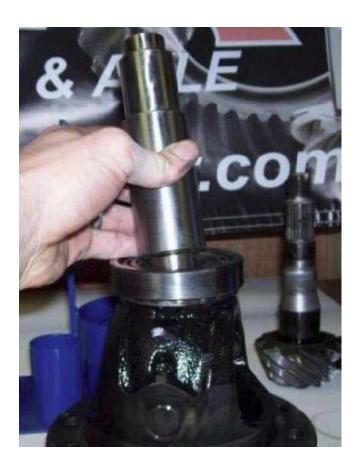
Place body of puller over adapter and screw bottom adjuster down onto race, slide clamshell half on and screw top adjuster until it contacts clamshell.
