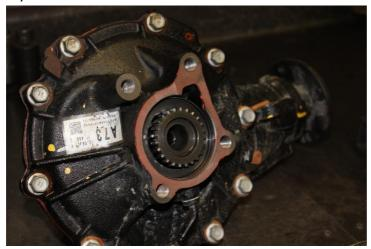
2. Using two pry bars or large screw drivers, apply upward force on the stub shaft. They do not come out easily; a decent amount of force must be applied to release the stub shaft.
