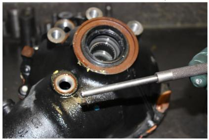
3. Slide the punch past the cross shaft and onto the stub shaft
