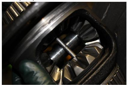
4. With a hammer tap the end of the punch until the stub shaft pops loose
