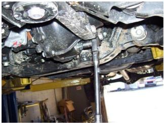
Separate Tie rod ends, a cheap tierod separator can be purchased or rented from an auto parts store or alternately one can use a hammer and give a good smack to the spindle tierod body. Tie rod separator is easy and cheap, do not use a fork tool you will ruin the boot.
