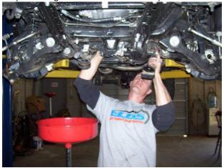
To remove the stub shaft for the ADD tube you can either use two pry-bars on either side or stick a small punch through the carrier from the drivers of the clamshell and tap it with a hammer.
