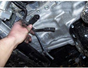
Now time to remove the mounting bolts and drop the diff, remove the allen nut 17mm, and the other 2 bolts as pictured. Remove allen nut completely remove one bolt completely, and back out last bolt almost all the way out, so diff is still hanging, diff will be rotated forward/down.
