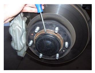
Remove Cotter pin and lock retainer:
