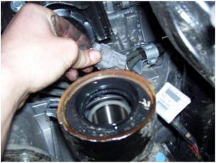
I like to go ahead and loosen the ADD tube retaining bolts, these are fairly tight and with the diff installed its a reasonable holding fixture. The tube can be fully removed now as well. But the tube serves as a useful place to grab when removing diff, and retains a bit of diff fluid that will surely drain all over you when you remove. I like to just break the bolts loose and leave it attached until it's on the bench.
