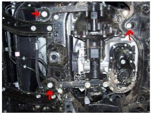
Position self to support and remove diff, rotate diff back up and remove last bolt while supporting diff, allow diff to rotate down and raise up until rear allen mount stud is free and lower. The 05+ diffs have more room than the early truck to get the diff out so that is a plus. Diff can be removed by one person and only ways about 55-60lbs.
