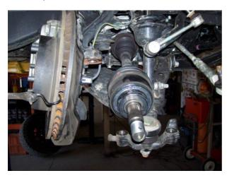
Remove CV shafts- use a pry bar to pop shaft out of tube and diff. internal c-clip is holding shaft in. A big brass drift can also be placed where prior bar is placed and can be knocked out with a hammer. I actually used the drift method as there is a metal dust seal on inner side of shaft that slightly interferes with pry method.
