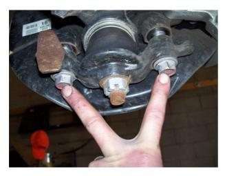
The spindle is now ready to be pulled away from the axle shaft giving you room to swing it out away from the CV, this allows for CV removal. The splines of the CV can be fairly seized in the internal hub splines. Screwing the axle nut back on shaft and popping the end of it, with a dead bow will free it up.
