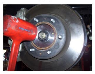
Getting the spindle away from the shaft is much easier with an assistant but possible by yourself, pull rotor spindle assembly away while pulling CV shaft back towards diff
