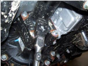
There is a 12mm bolt on top of the diff that holds the diff breather and vacuum line retainer bracket go ahead and back this bolt out and disconnect the two lines.
