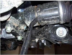
Unplug ADD motor harness careful not to break the plastic securing clips after all this is a 05+ truck let's keep it NEW!
