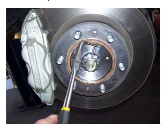
Remove axle nut 36mm w/ impact gun my battery powered electric took these off, if they are stuck or don't have power tools have an assistant hold the brakes while you put a breaker bar on it, if no assistant is available the nut can be broken loose by setting the tires on the ground in park and using a breaker bar, this should be done early on
