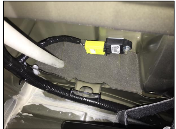
Figure 3. No. 5 Pillar Pad Installed
