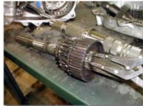
(Fig. 12) Front Drive Chain & Shaft Removal
