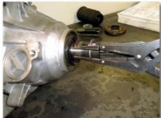
(Fig. 4) Stop Spacer & Snap Ring Removal
