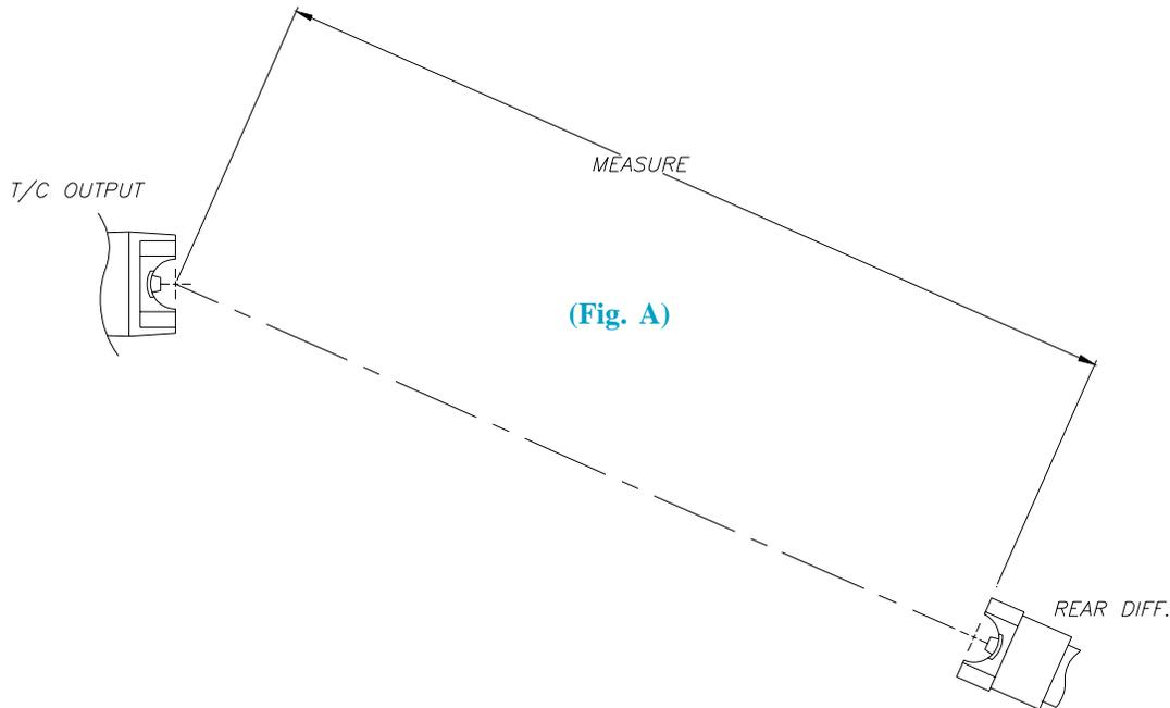
For proper C.V. type drive shaft operation, the rear differential should be pointed at the transfer case output yoke under normal driving load.
