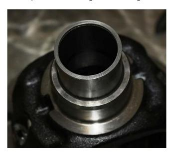
B. Install bushing flush with carrier (Be careful not to drive the bushing past flush as the design of the bushing is longer than the stock needle bearing to provide more support, however if driven to much past flush it will contact the spider gear)
