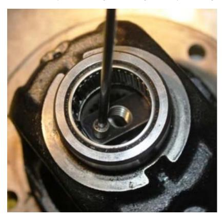
C. Once the Insert is installed thread the puller rod into the insert. Position insert parallel to ground, Pull out on puller rod to hold insert against bearing so that it is centered. (by placing the insert parallel if the tool slips down slightly do to gravity it still should not interfere with inside of carrier)
