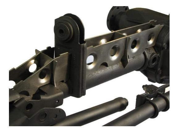
STEP 3. Using a marker or paint pen, indicate the areas on the axle where the truss touches the axle to prepare for welding. Remove truss pieces from axle. Using an angle grinder with either a flapper disc or wire wheel brush, clean the surface of the axle tube, casting, upper control arm mount, and coil perch until bare steel is exposed. Clean surfaces on drivers side casting, tube, and coil perch in a similar fashion.
